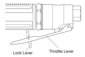
2 Hold the tool and while pressing the Lock Lever (1), press the Throttle Lever (2)
